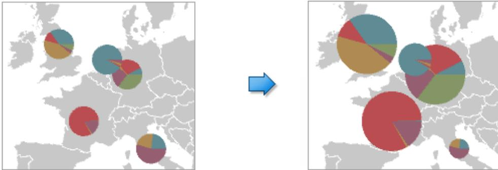
To enable this capability, use the Weighted Pies button in the Design ribbon tab.
